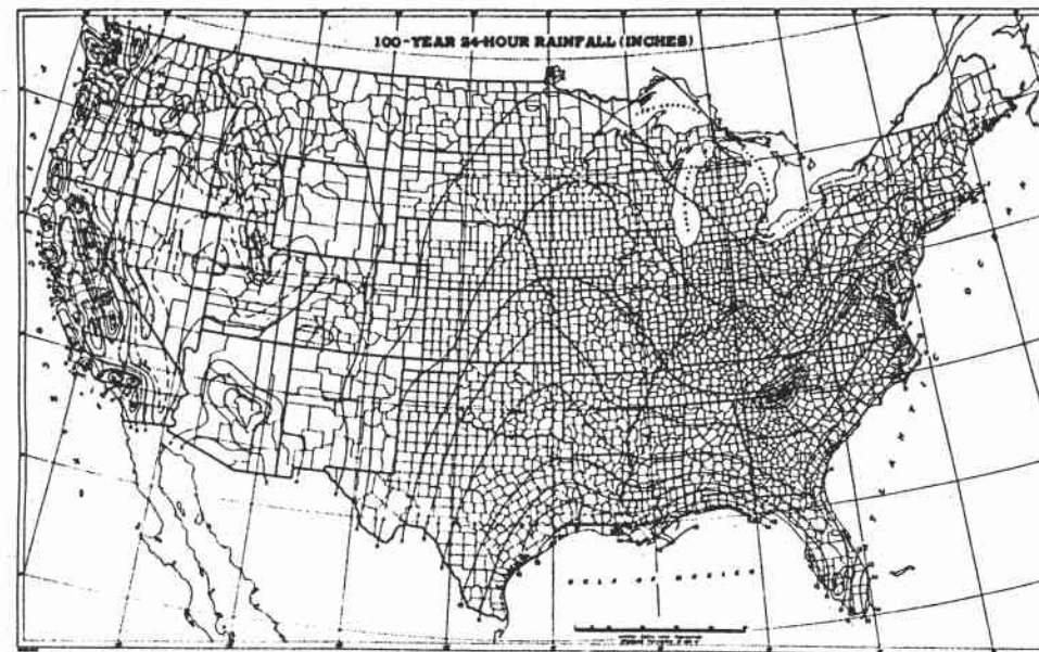
FIGURE 14.1.1 The 100-year 24-hour rainfall (in) in the United States as presented in U. S. Weather Bureau technical paper 40. (Source: Hershfield, 1961.)
