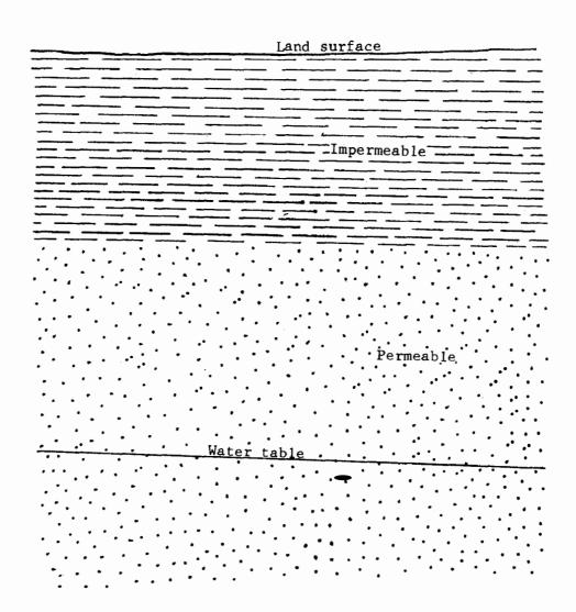
An impermeable or slowly permeable formation overlying an aquifer reduces or prevents natural recharge locally. The need for recharge is indicated by increased pumping lifts. The method of recharge is through injection wells. It may be possible to integrate surface drainage and recharge. Water quality may be a problem.
